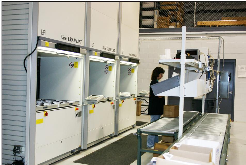
Orders are sent to the system and displayed on a monitor at the operators station. The screen directs the operator to the appropriate lift where an overhead LED display quickly directs them to the correct location on the provided tray and the correct quantity of the part.
